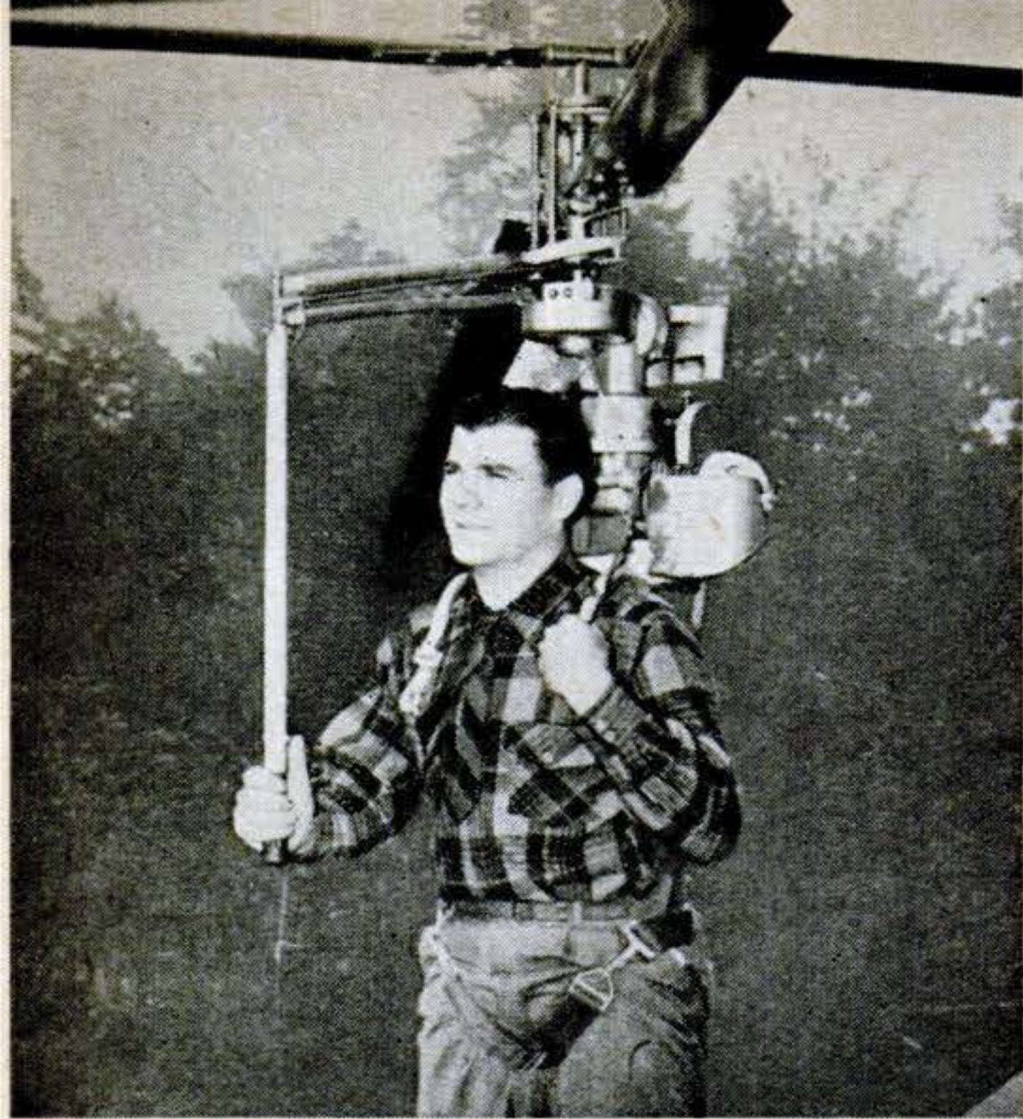
THE HOPPICOPTER , earlier back-pack rig, weighed only about 60 pounds, but its two-cylinder, 20-horsepower engine wasn't able to lift a man more than a few feet.
